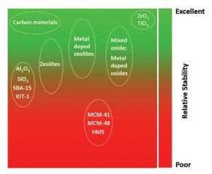
**Fig. 26** Hydrothermal stability of different heterogeneous solid catalysts in superheated steam conditions ( $T>400\,^{\circ}$ C). Reproduced with permission from ref. 284. Copyright (2014) Royal Society of Chemistry.
