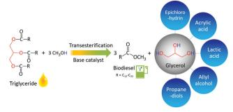
Fig. 10 Catalytic transformation of triglycerides (oils and fats) to produce biodiesel with glycerol as a byproduct, which can be upgraded to a variety of drop-in chemicals.
