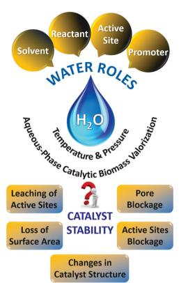
Fig. 33 Importance of water in liquid phase biomass valorization and its impact on catalyst stability.
