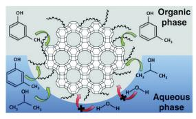
Fig. 34 The behavior of hydrophobized zeolites, prepared by silylation approach, in aqueous and organic phases. Reproduced with permission from ref. 490. Copyright (2012) American Chemical Society.
