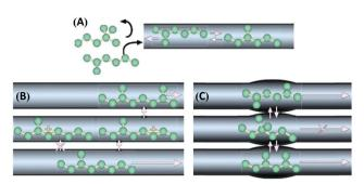
Fig. 6 Different types of shape selectivity in zeolites: (A) reactant shape selectivity, (B) transition state shape selectivity, and (C) product shape selectivity. Reproduced with permission from ref. 50. Copyright (2008) Springer Nature.
