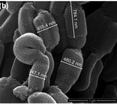
Fig. 20 SEM images of SBA-15-SO<sub>3</sub>H catalyst. Reproduced with permission from ref. 196. Copyright (2014) John Wiley and Sons.
