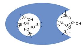
Fig. 12 Schematic representation of Zr grafting by treatment of dealuminated zeolites with  $ZrOCl_2$  in DMSO. Reproduced with permission from ref. 124. Copyright (2016) John Wiley and Sons.
