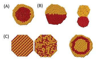
Fig. 24 Schematic representation of some possible mixing patterns of nanoalloys: (A) core-shell, (B) subcluster segregated, (C) mixed, and (D) three shell. The pictures show cross sections of the clusters. Reproduced with permission from ref. 263. Copyright (2008) American Chemical Society
