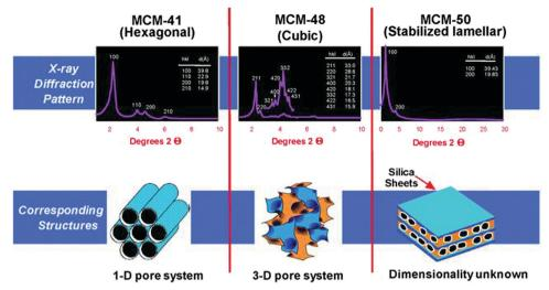
Fig. 17 Powder XRD patterns and structures of mesoporous SiO<sub>2</sub> materials (MCM-41, MCM-48, and MCM-50). MCM — Mobil Composition of Matter or Mobil Crystalline Material. Reproduced with permission from ref. 32. Copyright (2013) Royal Society of Chemistry.
