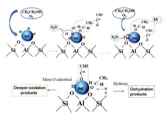
Fig. 13 Mechanism of ethyl acetate formation from ethanol through reverse hydrogen spillover process and the mechanism of dehydration and deeper oxidation over the Pd catalyst. Reproduced with permission from ref. 146. Copyright (2016) Royal Society of Chemistry.
