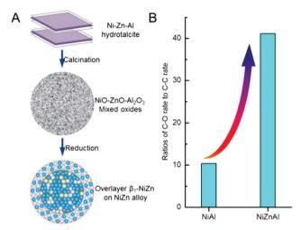
Fig. 28 (A) Structure evolution of NiZnAl catalyst and (B) comparison of reaction rates for C-O vs. C-C bond scission over NiAl and NiZnAl catalysts at similar HMF conversions. Reproduced with permission from ref. 345. Copyright (2017) American Chemical Society.
