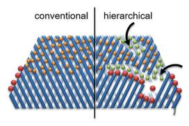
Fig. 14 Schematic representation of advantages of hierarchical zeolites towards active sites accessibility and transport/diffusion of reactants/ products. Reproduced with permission from ref. 8. Copyright (2016) Royal Society of Chemistry
