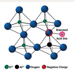
Fig. 5 Representative zeolite framework of a tetrahedral  $[SiO_4]^{4-}$ , with generation of a negative charge due to the incorporation of Al3+ and substitution of a proton to maintain the charge balance. Adapted with permission from ref. 45. Copyright (2002) Elsevier.
