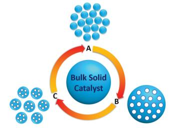
Fig. 3 Exemplary routes to improve surface area and diffusion properties of bulk solid catalysts: (A) reduction of particle size with shape-control, (B) introduction of pores, and (C) combination of both particle size reduction and introduction of pores.
