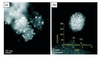
Fig. 27 Scanning transmission electron microscopic images of  $Pd-Pt/TiO_2$  catalyst at different magnifications. The formation of random Pd-Pt nanoalloys is confirmed from the Z-contrast high-angle annular darkfield imaging and the X-ray energy-dispersive spectrum (inset image, b) taken from an individual particle. Reproduced with permission from ref. 336. Copyright (2018) Royal Society of Chemistry.
