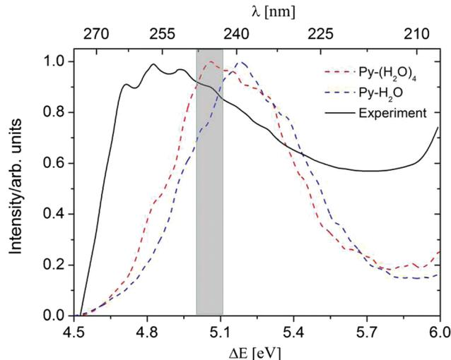
Fig. 2 Absorption spectra of the Py- $H_2O$  cluster (blue) and the Py- $(H_2O)_4$  cluster (red), simulated at the ADC(2)/cc-pVDZ level. The black line is the experimental spectrum of pyridine in aqueous solution.<sup>38</sup> The initial conditions for excited-state dynamics simulations of both clusters are sampled from an energy window of  $5.06 \pm 0.05$  eV (marked in grey).
