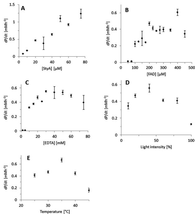
Fig. 1 Influence of some reaction parameters on the rate of the photoenzymatic epoxidation of styrene. General conditions (unless indicated otherwise in the figure): [styrene]<sub>0</sub> = 5 mM, [StyA] = 20 μM, [FAD] = 200 μM, [EDTA] = 20 mM, catalase = 600 U ml<sup>-1</sup>, [DMSO] = 1.25% (v/v), 100 mM KPi buffer (pH 7), 30 °C, stirring at 300 rpm, light intensity of 20% for 1 h. Error bars show the standard deviation for three independent experiments.
