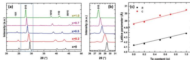
Fig. 4 (a) XRD patterns of as-deposited  $\text{Bi}_2(\text{Se}_{1-x}\text{Te}_x)_3$  films with  $x$  ranging from 0 to 1; (b) expanded XRD patterns showing the systematic shift of the 015 peak; (c) refined lattice parameters (see Table S1, ESI $^\dagger$ ) as a function of the Te content for different as-deposited  $\text{Bi}_2(\text{Se}_{1-x}\text{Te}_x)_3$  films.
