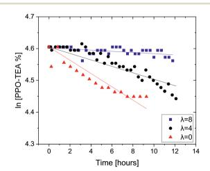
Fig. 2 Remaining PPO-TEA fractions as a function of time with hydration number  $\lambda = 0$ , 4 and 8, in 0.06 M OH<sup>-</sup> DMSO-d<sub>6</sub> solutions. All tests were done at room temperature.
