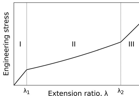
Fig. 1 The semi-soft elastic load curve as for a monodomain nematic LCE stressed perpendicular to the director. Curve was generated using equations of SSE theory taken from Warner and Terentjev.<sup>11</sup>
