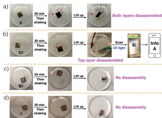
Fig. 4 Photographs of the double layer construct made up from Code B and Code A before and after immersion into chloroform solutions containing various anion salts (a) TBAF, (b) TBACl, (c) TBABr, and (d) TBAI for 20 min. The same concentration (20 mM) and volume (20 mL) were used for all experiments. The size of the substrate is 2.5 cm × 2.5 cm.
