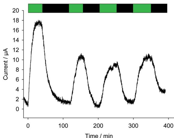
**Fig. 9** Four successive photocurrents as a function of time (after subtraction of the baseline) under green light pulses ( $\lambda = 530 \text{ nm}$ ; green bands) with a suspension of *Chlamydomonas reinhardtii*  $\Delta\text{petA}$  mutants ( $10^7$  cells per mL) in the presence of PPBQ ( $100 \mu\text{mol L}^{-1}$ ) after a pre-incubation time of 1 h.
