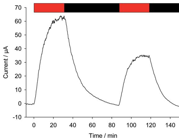
Fig. 2 Current as a function of time (after subtraction of the baseline). Two successive red light pulses have been applied ( $\lambda = 640$  nm;  $340 \mu\text{E m}^{-2} \text{s}^{-1}$ ;  $t = 30$  min: red rectangle) to a suspension of *Chlamydomonas reinhardtii* ( $\Delta\text{petA}$  mutants;  $10^7$  cells per mL) in the presence of 2,6 DCBQ ( $100 \mu\text{mol L}^{-1}$ ).
