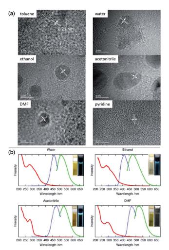
Fig. 3 Morphological characterization and optical studies: (a) high resolution transmission electron microscopy (HRTEM) images, (b) the normalized optical absorption spectra (red curve), photoluminescence excitation (blue curve) and photoluminescence emission (green curve) spectra of the carbon dots prepared by solvothermal methods with HATU in toluene, water, ethanol, acetonitrile, N,N-dimethylformamide (DMF) and pyridine, respectively.
