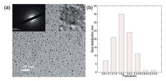
Fig. 4 Improved crystallinity and monodispersity due to metal ionic doping: (a) transmission electron microscopy (TEM) image with inset images of the selected area electron diffraction (SAED, left) and the high-resolution TEM image (right), and (b) the size distribution calculation based on one hundred dots of ACD-HATU doped with Al.
