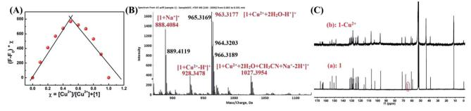
Fig. 7 (A) Job's plot for the complexation of 1 with  $Cu^{2+}$ , indicating the formation of a 1:1 complex. The total [1] +  $[Cu^{2+}] = 40 \mu M$ . (B) ESI-MS spectrum of 1-Cu<sup>2+</sup>. (C) <sup>13</sup>C NMR spectra of 1 upon addition of Cu<sup>2+</sup> in CD<sub>2</sub>Cl<sub>2</sub>.
