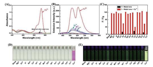
Fig. 1 Spectroscopic changes of  $1 (20 \,\mu\text{M})$  with the addition of various metal ions in CH<sub>3</sub>CN-H<sub>2</sub>O (9/1, v/v) solution. (A) Absorption spectral changes. (B) Fluorescence emission intensity changes. (C) The fluorescence intensity changes at 610 nm (black bars: 1 with other ions, red bars: 1 with Cu<sup>2+</sup> and other metal ions). (D) The color image with the addition of various metal ions. (E) The fluorescence image with the addition of various metal ions.
