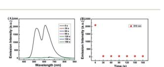
Fig. 5 (A) Time-dependent fluorescence intensity changes of sensor  $1-Cu^{2+}$  to  $H_2S$  in  $CH_3CN-H_2O$  (7/3, v/v) solution. (B) Relative fluorescence intensity at 610 nm as a function of time in  $CH_3CN-H_2O$  (7/3, v/v) solution.
