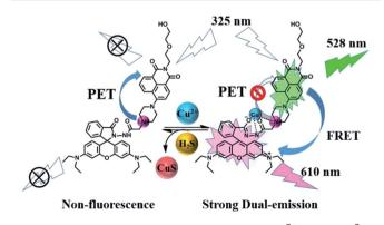
Fig. 9 The proposed mechanism of 1 to sense Cu<sup>2+</sup> and 1-Cu<sup>2+</sup> to sense H<sub>2</sub>S.
