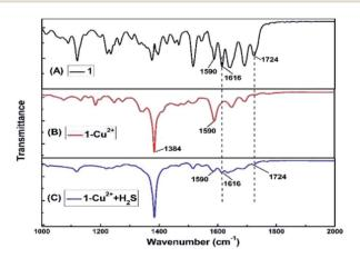
Partial FT-IR spectra of 1 (A),  $1-Cu^{2+}$  (B) and  $1-Cu^{2+} + H_2S$  (C).
