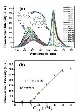
Fig. 7 (a) Fluorescence response of L (20  $\mu$ M) upon addition of PA from 10 to150  $\mu$ M (inset, the proposed structure of the spiro-lactam ring-opening product); (b) linear fitting analysis ( $\lambda_{ex}=314$  nm,  $\lambda_{em}=586$  nm) of the fluorescence intensity at 586 nm *versus* the concentration of PA.
