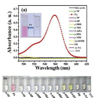
Fig. 3 (a) Absorption spectra of L (20  $\mu$ M) in the presence of various phenols (200  $\mu$ M) or NCAs (200  $\mu$ M); (b) corresponding photographs.
