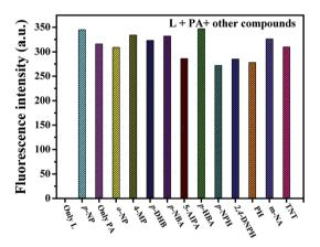
Fig. 5 Interference tests for probe L ( $\lambda_{ex}$  = 314 nm,  $\lambda_{em}$  = 586 nm, slits: 2.5 nm/5 nm).
