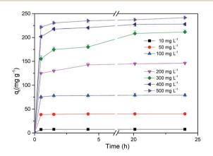
Fig. 5 The effect of contact time on the adsorption capacity at different initial MB concentrations (W = 0.025 g, V = 20 mL, T = 25 °C).
