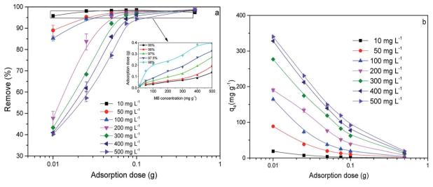
Fig. 4 The effect of different adsorption doses (T = 25 °C, t = 80 min).
