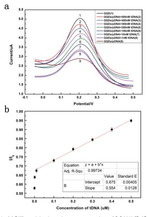
Fig. 6 (a) Differential pulse voltammograms plots of 0.2 M K<sub>3</sub>[Fe(CN)<sub>6</sub>] at pDNA (500 nM) immobilized GQDs modified GCE in 1.0 M KCl and that after hybridization with different concentrations of HBV-DNA (tDNA). (b) The plot of the peak current against the concentration of HBV-DNA.
