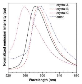
PL spectra of crystals A-C and an amorphous solid of PPQE.
