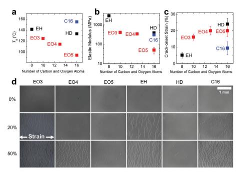
Fig. 1 Thermal and mechanical properties of the synthesized polymers. (a)  $T_g$ , (b) elastic modulus, and (c) crack-onset strain as functions of the number of carbon and oxygen atoms in the side chain. (c) Optical micrographs of the cracking behavior on PDMS at 0% (pristine), 20%, and 50% applied strain.
