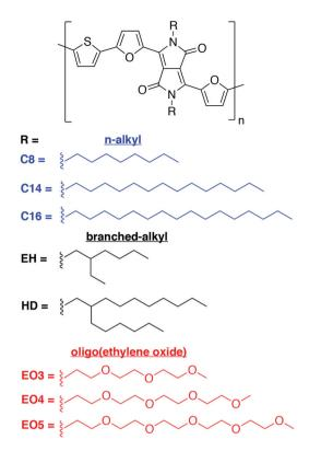
Scheme 1 Chemical structure of PDPP2FT polymers with linear (n-) alkyl, branched alkyl, and oligo(ethylene oxide) side chains. The polymers bearing *n*-alkyl side chains with 8 and 14 carbon atoms were obtained in low yields and with low molecular weights and were thus not studied further.
