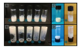
Fig. 2 Photographs of colloidal gels obtained by combining A01 and V01 at equal weight percent. (A) Taken with vials upright 2 h after preparation, (B) taken 20 min after inversion. Particle concentration: (a) 5 wt%; (b) 10 wt%; (c) 15 wt%; (d) 20 wt%; (c) 25 wt%. Also shown are individual latex solutions at 25 wt%: (f) A01 and (g) V01. (C) Upright, (D) taken 20 min after inversion.
