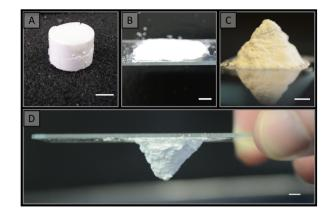
Fig. 9 Photographs of rigid porous materials obtained in a variety of formats from the addition of APS to V02 with 30 wt% DEGDA (w.r.t. solids). (A) Cylinder; (B) flat sheet; (C) & (D) pyramid. Scale bar is 5 mm.
