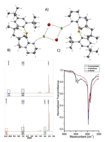
Fig. 2 (A) ORTEP representation of 2·H<sub>2</sub>O. Ellipsoids are plotted at 50% probability levels. (B) <sup>1</sup>H-NMR spectra of 2 and 2 + H<sub>2</sub>O. Top: Anhydrous. Bottom: H<sub>2</sub>O titrated 2. Red and blue box: N-H signal, green box: H<sub>2</sub>O signal shifted due to the presence of HB. Bottom integrals assume a dimeric species. (C) FTIR: -OH region expansion of 2 and 2 + H<sub>2</sub>O experiments (ESI/Fig. S6†).
