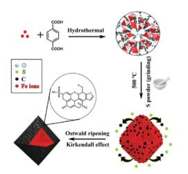
Fig. 28 MOF-templated strategy for the design of Fe/C-S catalysts. Reproduced with permission from ref. 263. Copyright (2017) Royal Society of Chemistry
