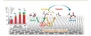
Fig. 12 Glycerol conversion and product yields as well as the proposed reaction pathways in glycerol hydrogenolysis over Cu-Pd/r-GO catalysts. Reproduced with permission from ref. 139. Copyright (2013) American Chemical Society
