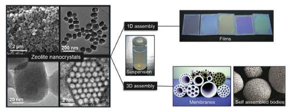
Fig. 2 Zeolite nanocrystals with diverse morphologies and sizes in colloidal suspensions and examples of processed forms as self-supported shapes, porous membranes, and optical quality films. Reproduced from ref. 64 S. Mintova, J. Grand and V. Valtchev, C. R. Chim., 2016, 19, 183-191. Copyright (c) 2016, published by Elsevier Masson SAS. All rights reserved.
