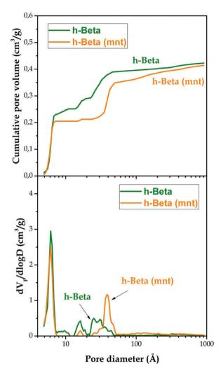
Fig. 5 Cumulative pore volume curves (upper graph) and pore size distribution curves (lower graph) of the h-Beta and h-Beta (mnt) samples obtained using the NLDFT method to analyse Ar adsorption-desorption isotherms measured at 87 K. Reprinted with permission from ref. 143
