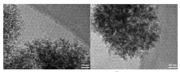
Fig. 3 TEM images of hierarchical ZSM-5 prepared using organosilanes in the synthesis gel.<sup>133</sup>
