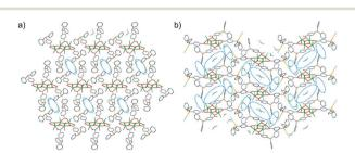
Fig. 3 a) Ladder-type packing of 1 and b) brick wall molecular arrangement of 2 (view along the crystallographic a-axis). The CH<sub>2</sub>Cl<sub>2</sub> solvent molecules are marked with dotted ice-blue line. The hydrogen atoms are omitted for clarity.
