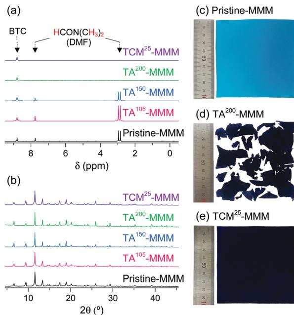
**Fig. 18** (a)  $^1\text{H}$  NMR spectra and (b) PXRD patterns of pristine-, TA<sup>105</sup>-, TA<sup>150</sup>-, TA<sup>200</sup>-, and TCM<sup>25</sup>-MMM. Photographs of (c) pristine-MMM, (d) TA<sup>200</sup>-MMM, and (e) TCM<sup>25</sup>-MMM. Reprinted (adapted) with permission from ref. 70. Copyright (2018) American Chemical Society.
