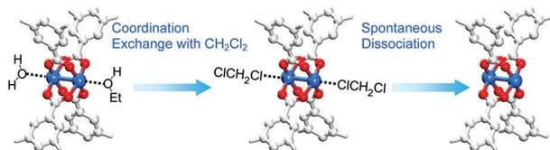
Fig. 3 Schematics illustrating activation of the paddle wheel-like ( $\text{Cu}^{\text{II}}_2$ ) node within HKUST-1 by DCM. Hydrogen atoms bound to carbon atoms in the benzene moieties are omitted for clarity. Reprinted (adapted) with permission from ref. 68. Copyright (2015) American Chemical Society.
