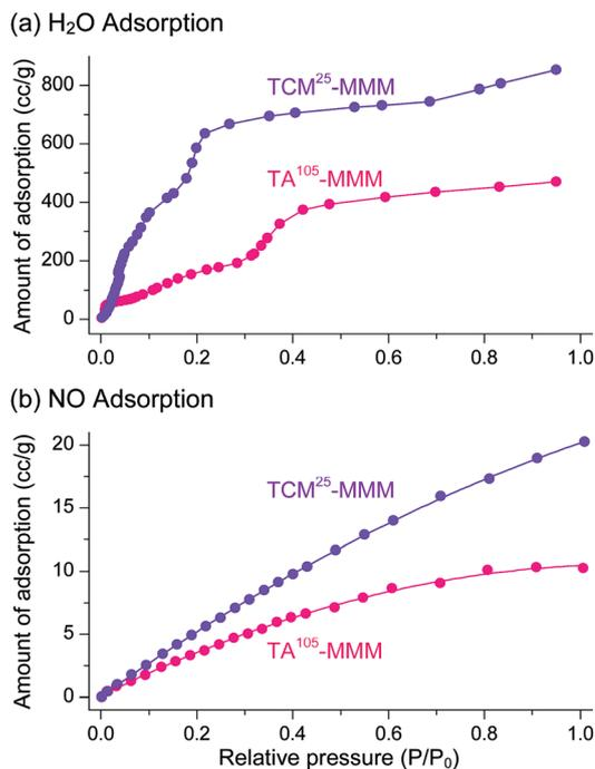
**Fig. 20** (a) H<sub>2</sub>O and (b) NO adsorption isotherms of TA<sup>105</sup>-MMM and TCM<sup>25</sup>-MMM. The isotherms for the TCM<sup>25</sup>-MMM sample were measured after applying vacuum at room temperature for 4 h. Reprinted (adapted) with permission from ref. 70. Copyright (2018) American Chemical Society.
