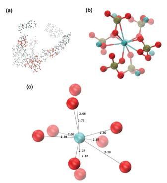
Fig. 10 Solution III: (a) aggregates after 5 ns; (b) detail of one of the Posner-like clusters formed with formula  $Ca_9(PO_4)_6$ ; (c) distances between the central Ca1 and the neighbouring oxygens. Colour key Ca: light blue, P: green, O: red, atoms not forming Posner's clusters: grey.
