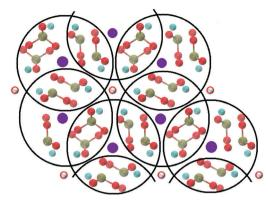
Fig. 2 Projection on the xy plane of crystalline HA, with Posner's clusters circled in black. Colour key Ca1: purple, Ca2: light blue, P: green, O: red,
