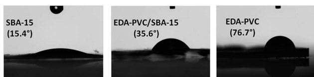
Fig. 9 Images from the contact angle measurement experiment on SBA-15, EDA-PVC/SBA-15 (4%) and unsupported EDA-PVC polymer.
