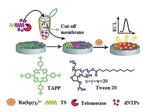
Fig. 5 Label-free electrochemiluminenscent detection of telomerase activity using porphyrin-functionalized graphene. Adapted with permission from ref. 41, Copyright 2012 WILEY-VCH Verlag GmbH & Co. KGaA. Weinheim
