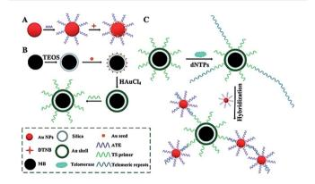
Fig. 6 SERS detection of telomerase activity using functionalized AuNPs and magnetic nanobeads. Adapted with permission from ref. 47, Copyright 2014 The Royal Society of Chemistry.
