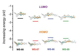
Fig. 4 Calculated frontier molecular orbitals (HOMO and LUMO) and energy gaps for dyes WS-66, WS-67, WS-68 and WS-69.
