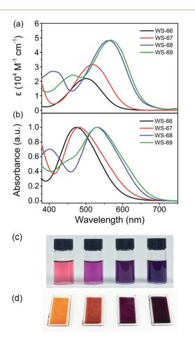
Fig. 2 Absorption spectra of dyes WS-66, WS-67, WS-68 and WS-69 in  $CH_2Cl_2$  (a) and on 3  $\mu$ m  $TiO_2$  films (b). Photographs of dyes WS-66, WS-67, WS-68 and WS-69 (from left to right) in solution (c) and on  $TiO_2$  films (d).
