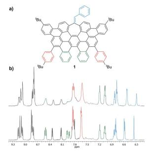
Fig. 2 (a) Structure of 1 and (b) partial <sup>1</sup>H-NMR spectra (500 MHz,  $C_2D_2Cl_4$ ) of **1** at: 293 K (top) and 369 K (bottom).
