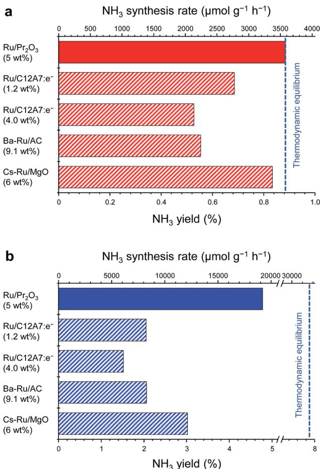
Fig. 1 Catalytic performance of supported Ru catalysts for NH<sub>3</sub> synthesis at (a) 0.1 MPa and (b) 1 MPa. Reaction conditions: catalyst, 0.2 g; reactant gas, H<sub>2</sub>/N<sub>2</sub> = 3 with a flow rate of 60 mL min<sup>-1</sup>; reaction temperature, 400 °C. With the exception of Ru/Pr<sub>2</sub>O<sub>3</sub>, NH<sub>3</sub> synthesis rates are reproduced from ref. 10.
