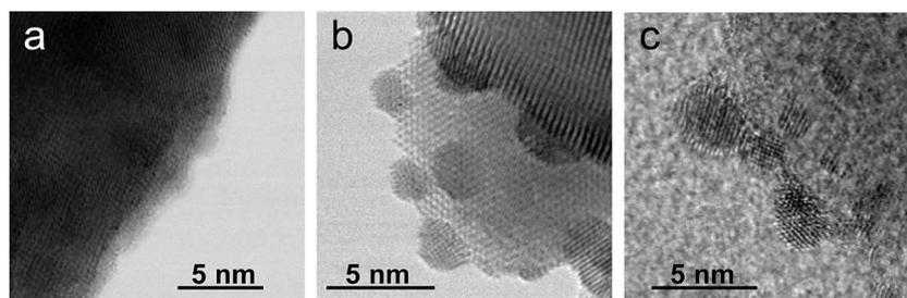
Fig. 4 HR-STEM images of (a) Ru/Pr<sub>2</sub>O<sub>3</sub>, (b) Ru/CeO<sub>2</sub>, and (c) Ru/MgO, after H<sub>2</sub> reduction.
