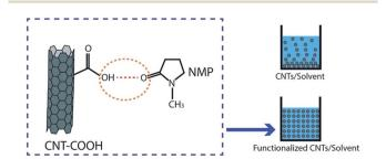
Fig. 3 Example of hydrogen bonding between functionalized CNT and solvent and the dispersion of functionalized CNT in the solvent.
