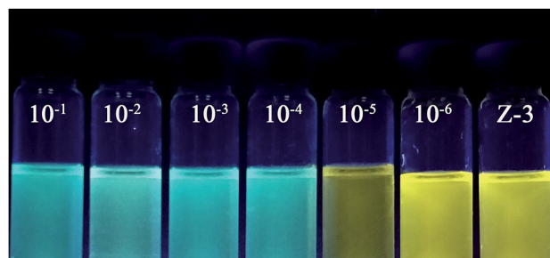
Fig. 6 Naked-eyes detection limit under UV lamp at 365 nm. From left to right, the concentration of \text{Hg}^{2+} is 10^{-1} M, 10^{-2} M, 10^{-3} M, 10^{-4} M, 10^{-5} M, 10^{-6} and 0 M.
