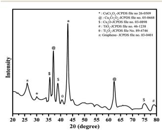
Fig. 1 XRD pattern of the synthesized catalyst.
