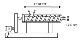
Fig. 7 Representation of a single-screw extruder.
