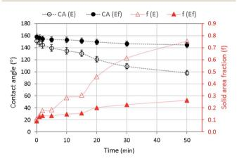
Fig. 6 LB contact angle (CA) and solid area fraction (f) for E and E<sub>f</sub> substrates as a function of time.
