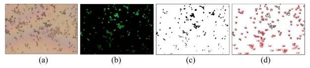
Fig. 4 Image analysis for measurement of an area fraction (%) covered by *E. coli*: (a) bright field image, (b) fluorescence image, (c) black and white binary image produced using ImageJ, (d) boundary of bacteria-covered area analyzed from (b) using ImageJ.
