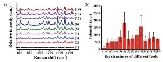
Fig. 9 (a) Raman spectra of R6G molecules on the structured Cu (110) substrate at a concentration of  $10^{-6}$  M with different machining velocities. (b) Average Raman intensity of the 1362 cm<sup>-1</sup> R6G peak of 20  $\mu$ m  $\times$  20  $\mu$ m of arrayed inverted pyramid cavities with different machining velocities.
