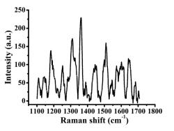
Fig. 11 Raman spectra of R6G molecules on the  $SiO_2$  substrate at a concentration of 0.25 M.
