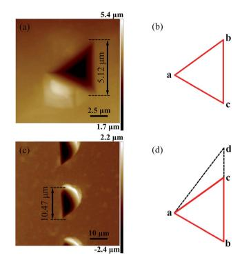
Fig. 3 (a) AFM images of the inverted pyramid cavity when the precision stage is fixed. (b) Schematic shapes of the cavity when the precision stage is fixed. (c) AFM images of the inverted pyramid cavity when the precision stage is moved. (d) Schematic shapes of the cavity when the precision stage is moved.
