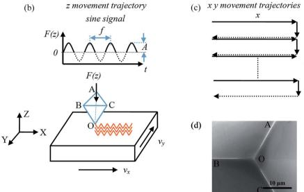
Fig. 1 (a) Schematic of the home-built tip-based force modulated indentation system. (b) Machining process for the fabrication of substrates with periodic micro/nano-cavities. (c) Movement trajectories of the x and y directions during machining. (d) SEM image of the cube corner tip with its shape.
