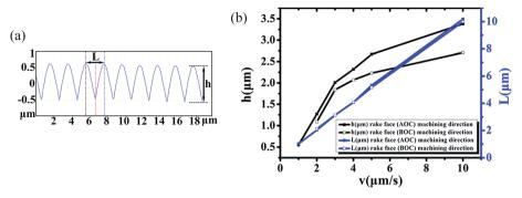
Fig. 6 (a) Schematic diagram of the depth and the width of cavities. (b) Relationship between the dimensions of the cavities and the moving velocity of the precision stage.
