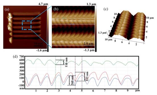
Fig. 10 (a) AFM images of arrayed inverted pyramid cavities machined with  $v_x = 5 \, \mu \text{m s}^{-1}$  and  $v_y = 1 \, \mu \text{m s}^{-1}$ . (b) Enlarged image of the local position of figure (a). (c) Three-dimensional view of structures with  $v_x = 5 \, \mu \text{m s}^{-1}$  and  $v_y = 1 \, \mu \text{m s}^{-1}$ . (d) Sectional view of the structures in figure (b).
