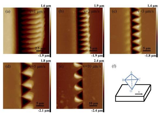
Fig. 4 AFM images of the arrayed inverted pyramid cavities with different machining velocities with the plane AOC of the cube corner tip as the rake face (a)–(e) the machining velocity of 2, 3, 4, 5 and 10  $\mu$ m s<sup>-1</sup>, respectively. (f) Schematic machining direction with the plane AOC of the cube corner tip.
