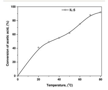
Fig. 3 Conversion of acetic acid into an ester with *n*-butanol as a function of reaction temperature using IL-5 at 90 min reaction time.
