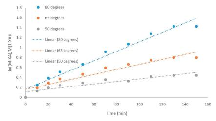
Fig. 5 Plot for the kinetic study of IL-5 at three different temperatures (50 °C, 65 °C, and 80 °C) in the time span ranging from 0 to 150 min.
