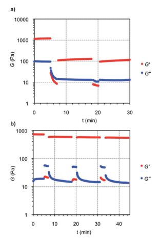
Fig. 12 Representative 3-steps loop rheological test for (a) GB hydrogel and (b) OxA-GB10 hybrid hydrogel.
