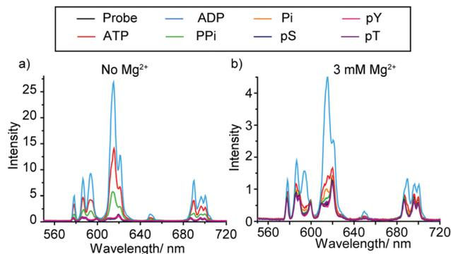
**Fig. 2** Change in emission spectra of **[Eu.1]**<sup>+</sup> (8  $\mu\text{M}$ ) in the presence of different phosphate anions (1 mM, sodium salts) in buffered aqueous solution (10 mM HEPES, pH 7.0), containing: (a) no  $\text{Mg}^{2+}$  ions; (b) 3 mM  $\text{Mg}^{2+}$  ions.  $\lambda_{\text{exc}} = 330$  nm, 298 K.
