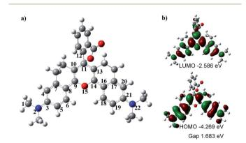
Fig. 4 (a) DFT optimized structure of HN7. In the ball-and-stick representation, carbon, nitrogen, oxygen, and hydrogen atoms are colored in gray, blue, red, and white, respectively. (b) Molecular orbital plots (LUMO and HOMO) and HOMO/LUMO energy gaps of HN7.
