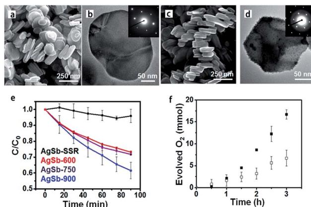
Fig. 7 (a) SEM and (b) TEM images of the  $\text{NaSbO}_3$  product obtained from an aerosol-assisted synthesis. (c) SEM and (d) TEM images of the  $\text{AgSbO}_3$ , single-crystalline  $\text{NaSbO}_3$  plates in molten  $\text{AgNO}_3$  were used as the template. (e) Rhodamine B photocatalytic degradation under  $\lambda = 400\text{--}500 \text{ nm}$  illumination. (f) Oxygen evolution in the presence of  $0.1 \text{ M AgNO}_3$  (ref. 55 Copyright 2015, American Chemical Society).
