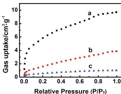
**Fig. 8** The adsorption curves of CO<sub>2</sub> (a), CO (b) and CH<sub>4</sub> (c) at 298 K on the Zn-MOF synthesized at  $x = 0.38$ .
