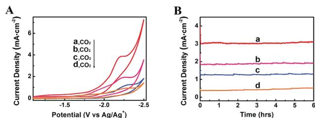
Fig. 6 CV traces (A) and current density profiles at an applied potential of -2.2 V vs. Ag/Ag<sup>+</sup> (B) using different kinds of ILs as electrolytes: (a) BmimBF<sub>4</sub>; (b) BmimOTf; (c) BmimPF<sub>6</sub>; (d) BmimClO<sub>4</sub>.
