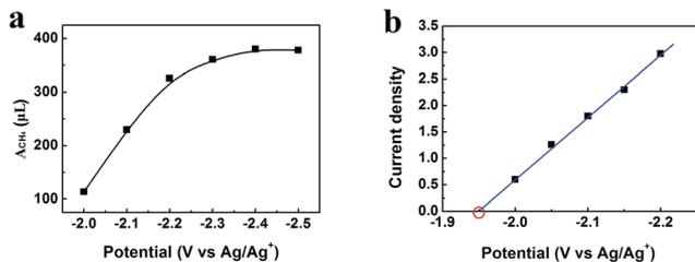
Fig. 5 (a) Amount of CH<sub>4</sub> ( $A_{\text{CH}_4}$ , volume at standard temperature and pressure) generated in 2 h under different potentials. (b) Current densities for CH<sub>4</sub> under different potentials and the equilibrium potential can be obtained by extrapolation method.
