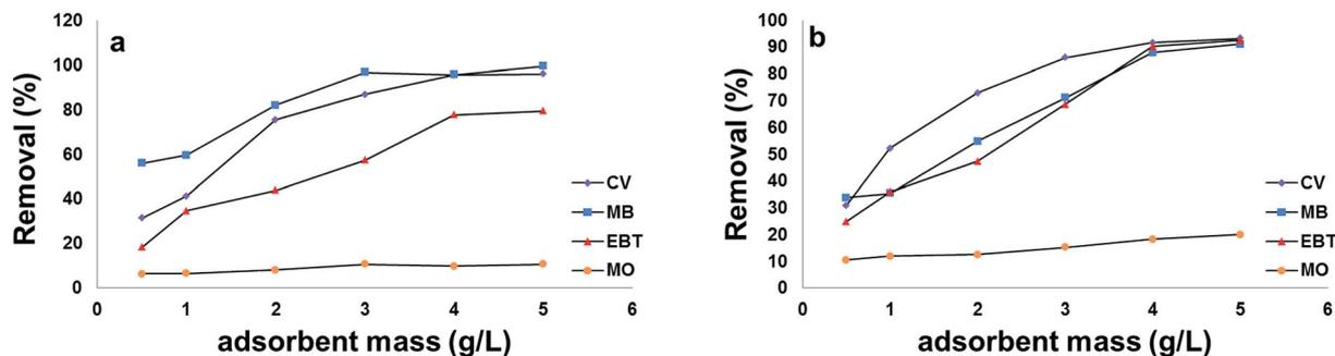
Fig. 9 Effect of adsorbent mass on the removal efficiency of model dyes onto: [a] MSP NPs and [b] MP NPs. Dyes  $100 \text{ mg L}^{-1}$ , temperature:  $25 \text{ }^\circ\text{C}$ , pH: 2.0 for anionic dyes and 8.0 for cationic dyes, time: 120 min. Magnetite/Pectin Nanoparticles: MP NPs and Magnetite/Silica/Pectin Nanoparticles: MSP NPs.
