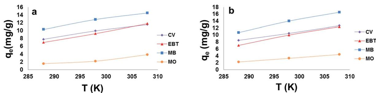
Fig. 10 Effect of temperature on the adsorption capacity ( $q_e$ ) of model dyes onto; [a] MSP NPs and [b] MP NPs. Adsorbent: 5 g L<sup>-1</sup>, dyes 10 mg L<sup>-1</sup>, pH: 2.0 for anionic dyes and 8.0 for cationic dyes, time: 120 min. Magnetite/Pectin Nanoparticles: MP NPs and Magnetite/Silica/Pectin Nanoparticles: MSP NPs.
