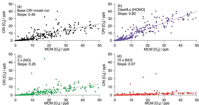
**Fig. 10** Correlation of CRI modelled [O<sub>3</sub>] from winter ClearLo IOP against MCM modelled [O<sub>3</sub>]. (a) Base CRI model, (b) CRI constrained to ClearLo measured HONO, (c) Base CRI model run, but with [NO] doubled, (d) Base CRI model run, but with [NO] increased tenfold. All data can be found in Table 5.
