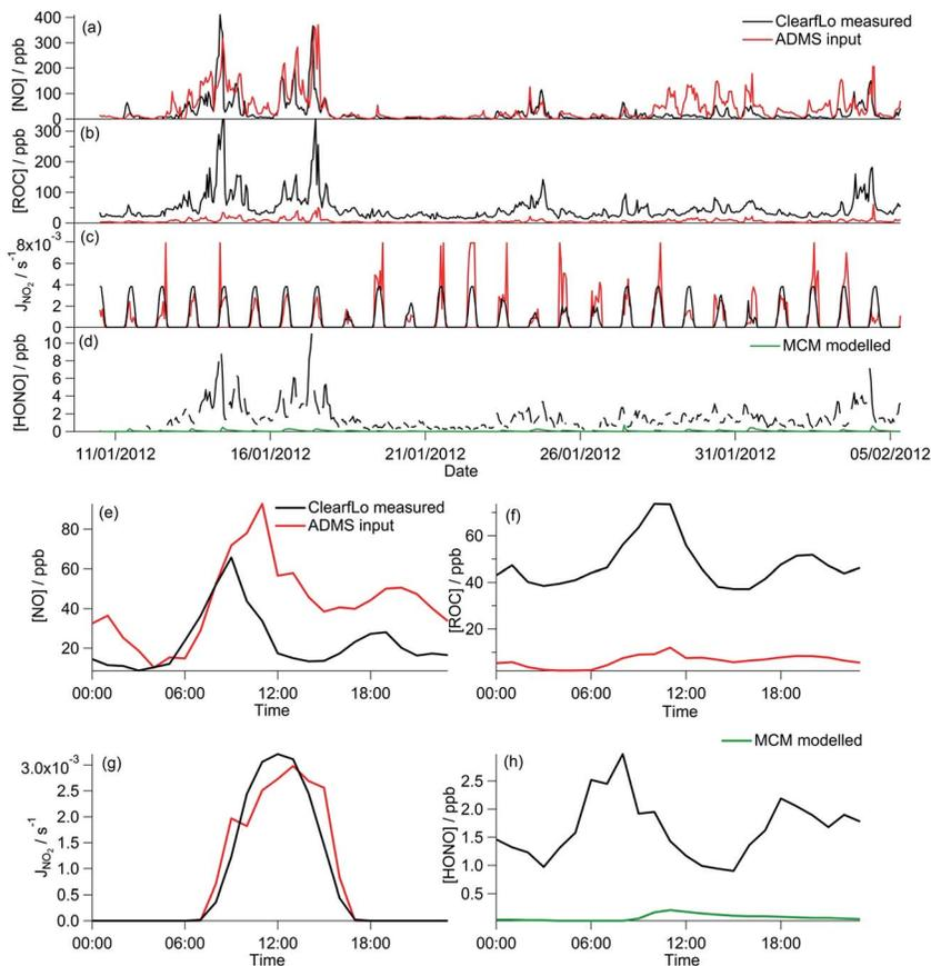
Fig. 8 (a–c) Full time series of ADMS-Urban inputs and measured NO and VOC concentrations and NO<sub>2</sub> photolysis frequency from ClearfLo winter IOP. (d) Full time series of MCM modelled HONO concentrations and ClearfLo measured HONO. (e–h) Average diurnal cycle of the time series in panels a–d.
