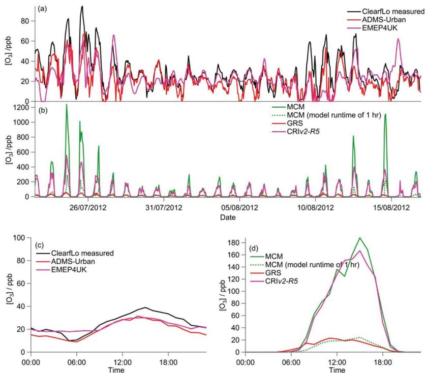
Fig. 3 (a) Full time series of ADMS-Urban, EMEP4UK modelled and measured  $O_3$  concentrations from ClearfLo summer IOP. (b) Time series of the ozone predicted by the chemistry schemes GRS, CRIV2-R5 and MCMv3.2 run in box models to steady state (MCM  $[O_3]$  predicted after 1 h model run time also shown) from ClearfLo summer IOP (c) corresponding median diurnal cycle profile from the data in panel (a). (d) Corresponding median diurnal cycle from the data in panel (b).
