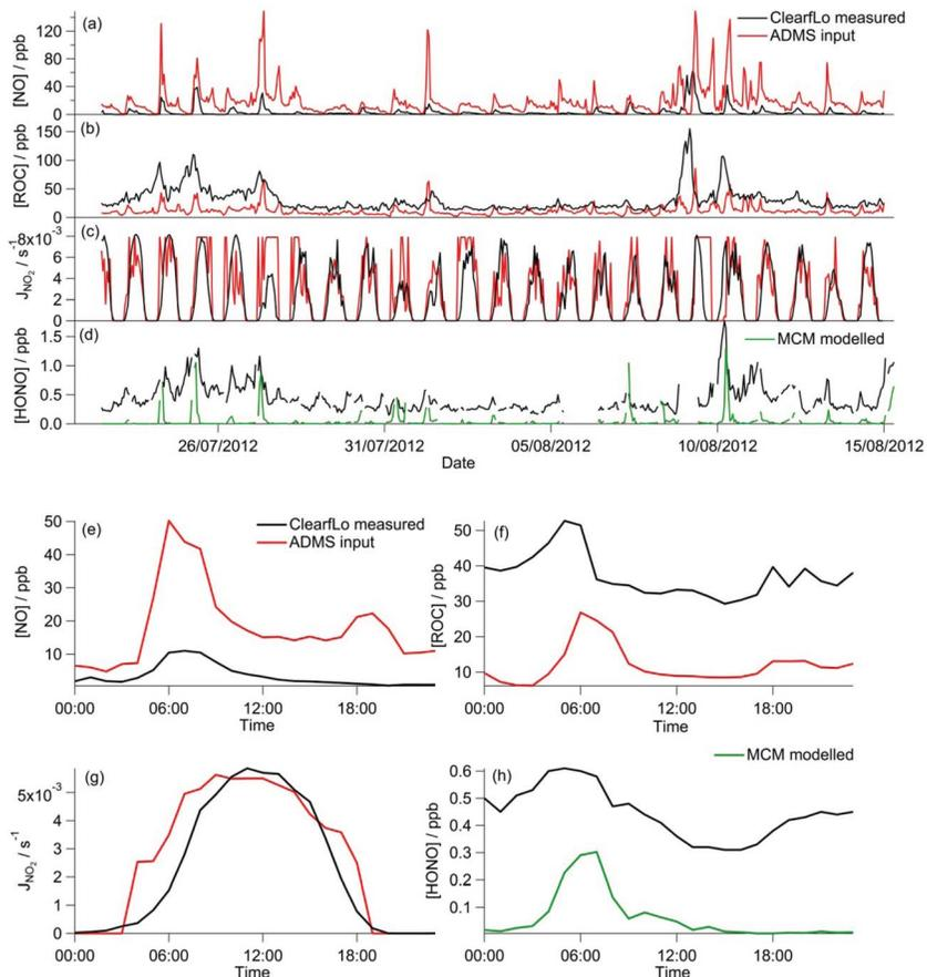
Fig. 4 (a–c) Full time series of ADMS-Urban inputs and measured NO and VOC concentrations and NO<sub>2</sub> photolysis frequency from ClearLo summer IOP. (d) Full time series of MCM modelled HONO concentrations and ClearLo measured HONO. (e–h) Average diurnal cycle of the time series in panels a–d.
