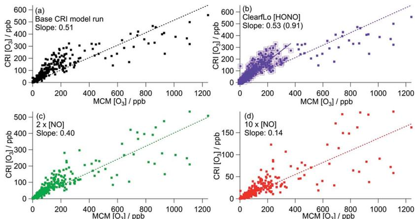
Fig. 6 Correlation of CRI modelled  $[O_3]$  from summer ClearfLo IOP against MCM modelled  $[O_3]$ . (a) Base CRI model run (value in parentheses = slope when MCM modelled  $[O_3]$  is <400 ppb). (b) CRI constrained to ClearfLo measured HONO. (c) Base CRI model run, but with  $[NO]$  doubled. (d) Base CRI model run, but with  $[NO]$  increased ten-fold. All data can be found in Table 3.
