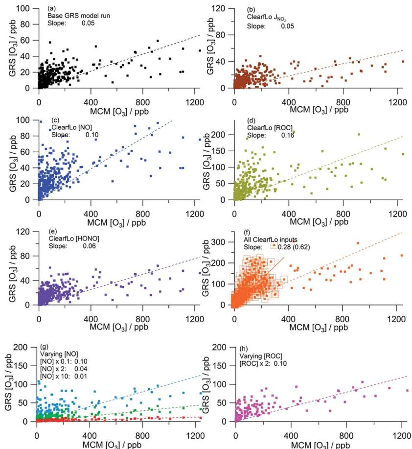
Fig. 5 Correlation of MCM modelled  $[O_3]$  from summer ClearfLo IOP against GRS modelled  $[O_3]$ . (a) Base GRS scheme, (b) ClearfLo measured  $j(NO_2)$ , (c) measured ClearfLo  $[NO]$ , (d) measured ClearfLo  $[ROC]$ , (e) measured ClearfLo  $[HONO]$ , (f) all ClearfLo measured data (value in parentheses = slope when MCM modelled  $[O_3]$  is <400 ppb), (g) & (h) varying  $[NO]$  and  $[ROC]$ . All data can be found in Table 2.
