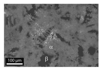
Fig. 2 Backscattered image of sample #5. Three different phases are clearly distinguishable: the main phase  $\alpha$ , the Mg<sub>2</sub>Si-like phase  $\beta$  and the Sn-rich phase  $\gamma$ . EDX analysis reveals that these phases show significant local concentration fluctuations
