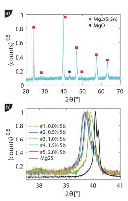
Fig. 1 (a) X-ray diffraction data of sample #2. All major peaks can be indexed as (shifted) Mg<sub>2</sub>Si peaks. Minor peaks for MgO can also be observed. (b) The zoom-in around the (220) peak reveals peak broadening and emphasizes the shift compared to the Mg<sub>2</sub>Si sample.
