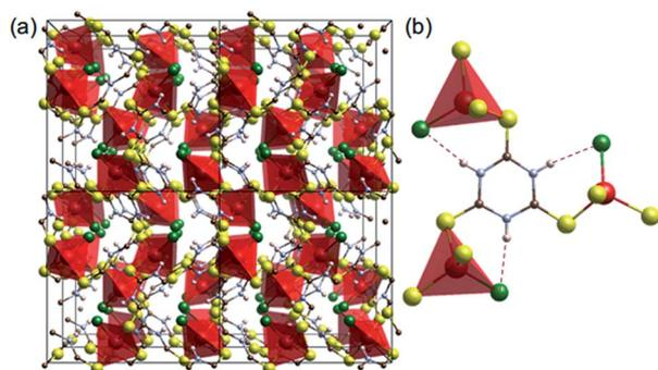
Fig. 1 Crystal structure of  $[\text{CuCl}(\text{ttcH}_3)]_{13}$ . (a)  $2 \times 2 \times 2$  cells. (b) Connectivity of  $\text{CuClS}_3$  tetrahedral with the thioketone form of tri-thiocyanuric acid molecules (red: Cu, green: Cl, yellow: S, blue: N, brown: C, and white: H). Dotted lines show hydrogen bonding.
