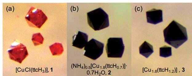
Fig. 2 Photos of (a) **1** CuCl(ttcH<sub>3</sub>) crystals, (b) **2** – *i.e.* **1** treated in aqueous ammonia for 2 days, and (c) **3** – *i.e.* **2** dried at 130 °C under vacuum. The large monoliths are about 100  $\mu$ m across.
