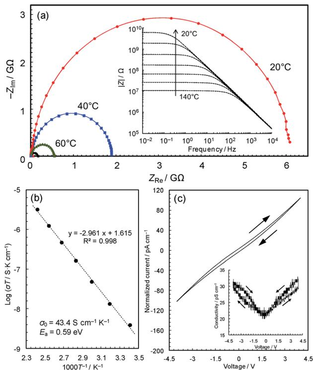
Fig. 3 AC impedance analyses. (a) Complex-plane impedance data for a pellet of **3** (red: 20 °C; blue: 40 °C; green: 60 °C; and black: 80 °C). The inset shows  $\log|Z|$  vs.  $\log$  frequency plots. (b) Arrhenius plot of the electronic conductivity. (c) Current–voltage characteristics measured by cyclic voltammetry scanned at 10  $\text{mV s}^{-1}$  at 25 °C.
