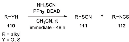
Scheme 39 Synthesis of thiocyanates and isothiocyanates with the thiocyanate anion as the nucleophile.
