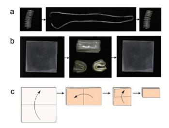
Fig. 11 Visual demonstration of the high strain capability for Epon1. (a) The shape memory and recovery steps of a tight spiral; (b) a square sample was folded three times and visualized in different directions; (c) the folding steps of the square sample.
