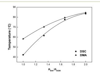
Fig. 4 Glass transition temperatures of the epoxy samples.
