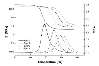
Fig. 3 DMA curves of the epoxy samples.
