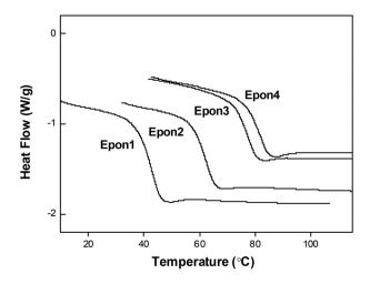
Fig. 2 DSC curves of the epoxy samples.
