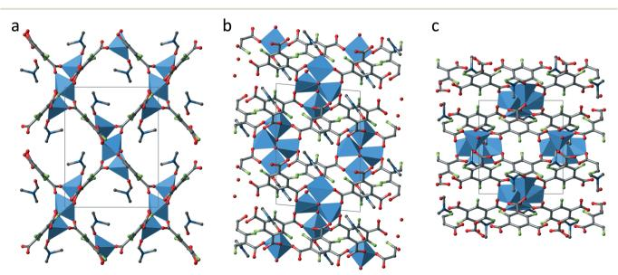
Fig. 3 Extended unit cell of UHM-32 along the a-axis (a), the b-axis (b) and the c-axis (c); grey: carbon, red: oxygen, blue: copper, green: fluorine, hydrogen atoms and solvent molecules (apart from the DMA molecules coordinated to the SBU) are omitted for clarity. The coordination spheres of the copper ions are illustrated by the blue polyhedra.
