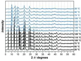
Fig. 6 Variable temperature powder XRD patterns of UHM-32 (top) and UHM-33 (bottom). The temperature was increased from 28 °C to 50 °C and 75 °C, than in steps of 10 °C up to 150 °C. The samples were than cooled down to room temperature in steps of 25 °C. Blue represents the new built phases.
