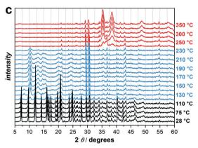
Fig. 5 Variable temperature powder XRD pattern of UMH-31 (a), UHM-32 (b) and UHM-33 (c). For each experiment 23 diffractograms were measured, the first three ones at 28, 50 and 75 °C, followed by temperature steps of 10 °C from 100 up to 250 °C and steps of 25 °C up to 350 °C. Black represents the original MOF phase, blue the new MOF phases and red the decomposition products. The two reflections at  $2\theta$  = 29.4 and  $2\theta$  = 30.5 are probably caused by the sample holder.
