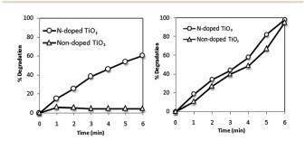
Fig. 4 Photocatalytic degradation of direct black 38 as a function of time under visible light (left) and sunlight (right). Experimental conditions:  $C_{\rm o}=0.055~{\rm g~L^{-1}}$ ,  $C_{\rm catalyst}=1.0~{\rm g~L^{-1}}$ , pH = 2.5,  $T=25~{\rm ^{\circ}C.^{153}}$
