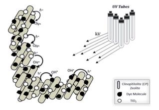
Fig. 8 Synergistic effect of TiO2 and clinopitilolite catalyst on dye degradation by producing OH free radicals.318
