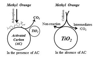
Fig. 9 Synergistic mechanism between  $AC-TiO_2$  composites. The arrow labelling un-reacted emphasizes that in the absence of Absorbent the reactants may remain un-reacted into the solution resulting in low photoactivity of methyl orange.<sup>236</sup>
