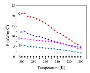
**Fig. 7** Temperature dependence of the power factor of prepared samples: (A) pure PEDOT:PSS nanofilm, (B) SWCNTs/PEDOT:PSS layered nanostructure, (C) SWCNTs/PEDOT:PSS (doped with DMSO) layered nanostructure, (D) SWCNTs/PSS layered nanostructure, (E) SWCNTs/PVA layered nanostructure.
