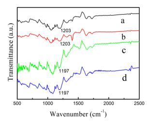
**Fig. 4** FT-IR spectra of prepared samples: (a) pure PEDOT:PSS, (b) PEDOT:PSS doped with DMSO, (c) SWCNTs/PEDOT:PSS layered nanostructure, (d) SWCNTs/PEDOT:PSS (doped with DMSO) layered nanostructure.
