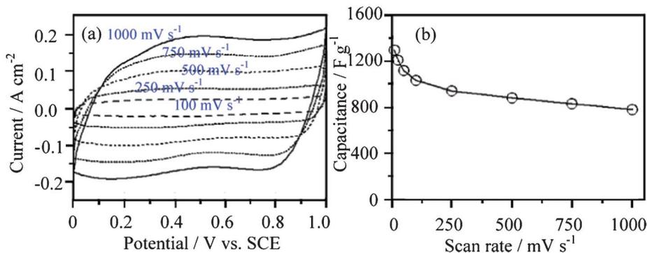
**Fig. 8** (a) CV curves at different scan rates and (b) dependence of the capacitance on the scan rate for an annealed RuO<sub>2</sub>·xH<sub>2</sub>O nanotube arrayed electrode (0.19 mg cm<sup>-2</sup>) in 1.0 mol l<sup>-1</sup> H<sub>2</sub>SO<sub>4</sub> solution (modified from ref. 54a).
