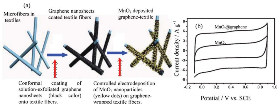
**Fig. 9** (a) Schematic illustration of two key steps for preparing hybrid MnO<sub>2</sub>-nanostructured textiles@graphene and (b) CV curves of an optimized MnO<sub>2</sub>@graphene at different potential windows at the scan rate of 20 mV s<sup>-1</sup> in 1 mol l<sup>-1</sup> Na<sub>2</sub>SO<sub>4</sub> solution (modified from ref. 8a and 8b, respectively).
