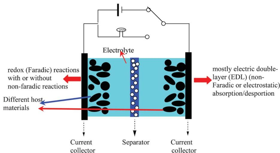
**Fig. 1** Schematic illustration of ASCs.
