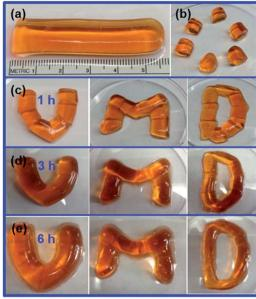
**Fig. 2** The use of the self-healing nature of the hydrogel to produce complex architectures. (a) The original hydrogel. (b) The hydrogel after being cut. (c–e) The hydrogel segments arranged in the form of letters: U, M, and D, after (c) 1 hour, (d) 3 hours, and (e) 6 hours of self-healing.
