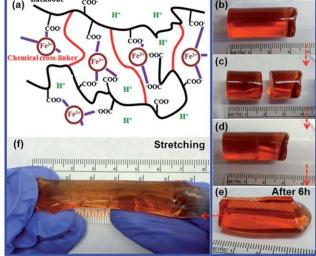
**Fig. 1** (a) Schematic illustration of the structure of the self healing hydrogel. (b)–(e) Self healing of a cylindrical hydrogel (Entry 3) at room temperature: (b) the original hydrogel, (c) the hydrogel after being cut, (d) the hydrogel after the two parts were brought into contact with each other, (e) the hydrogel after healing for 6 hours. (f) Stretching the self-healed hydrogel up to  $\sim$ 200%.
